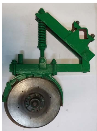
Figure 1 – Experimental disc coulters with suspension mechanism
